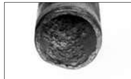
Figure CG-10. Oxygen in the system speeds corrosion (oxidation) of pipes, causing pitting such as shown here.
